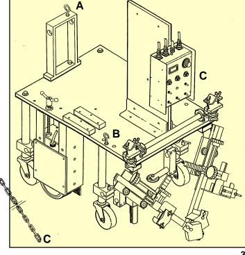
Continuous or intermittent welds: Weld length timer: 1-30 seconds
