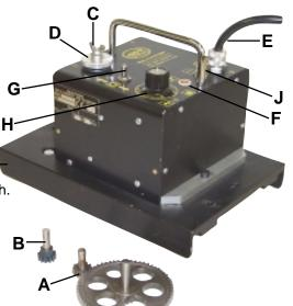
Two pinion gears are provided. The factory installed pinion engages the bull gear to provide a high torque, low speed range (A). The user can easily install the alternate pinion to bypass the bull gear and obtain a low torque, high speed range (B).
